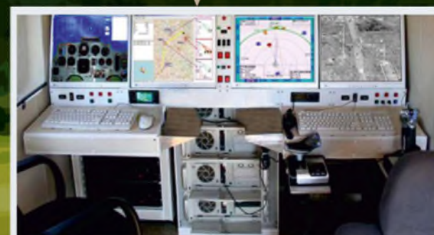
GROUND SYSTEM OF INFORMATION RECEIVING AND TRANSMISSION
